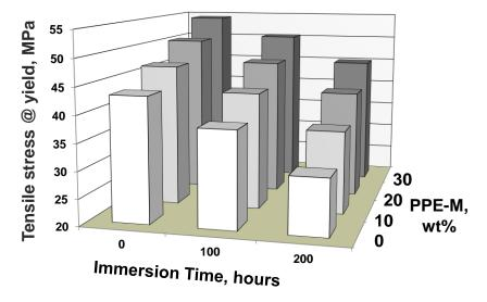
Figure 16. Tensile stress after immersion in water
