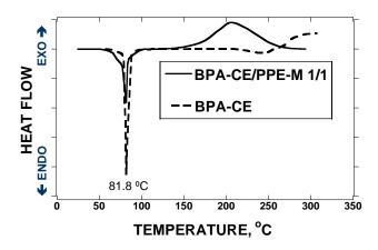
Figure 3. DSC curves of BPA-CE and BPA-CE/PPE-M
