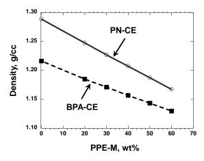
Figure 9. Density for BPA-CE/PPE-M and PN-CE/PPE-M
