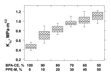
Figure 7. Fracture Toughness of BPA-CE/PPE-M
