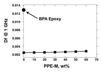
Figure 11. Loss Tangent for BPA-CE/PPE-M
