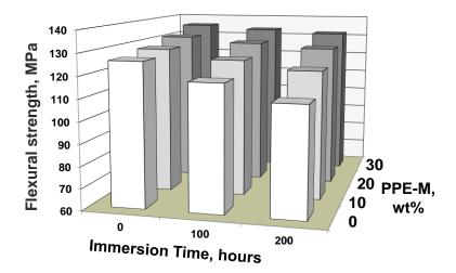
Figure 17. Flexural strength after immersion in water
