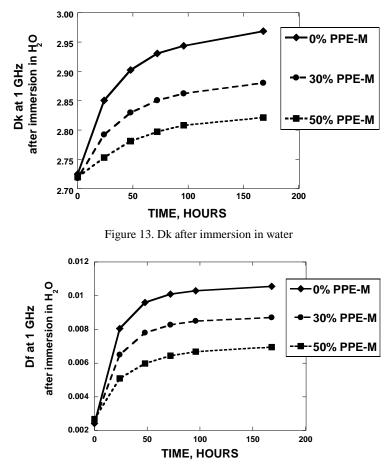
Figure 14. Dk after immersion in water
