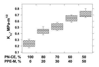
Figure 8. Fracture Toughness of PN-CE/PPE-M
