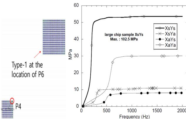
Figure 6. (a) Maximum solder stress location at Xs-Ys of the modified sample using 1/4 model. (b) The stress developments by changing the boundary conditions.
