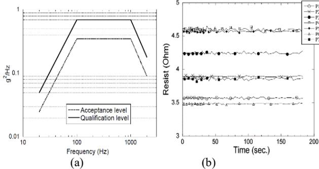
**Figure 2.** (a) Power spectrum densities of the two levels. (b) The solder resistance measurements during the qualification level.
