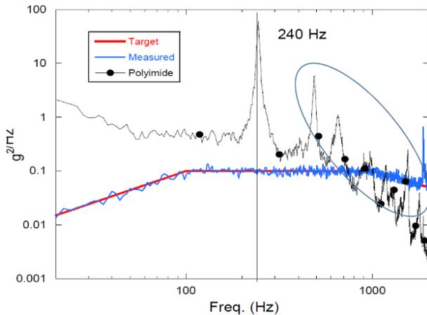
**Figure 3.** The PCB vibration behavior measurements under the random vibration.
