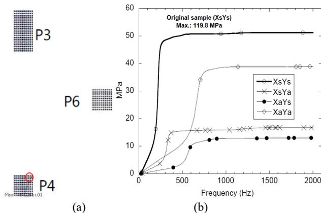
Figure 5. (a) Maximum solder stress location at Xs-Ys of the sample using 1/4 model. (b) The stress developments by changing the boundary conditions.
