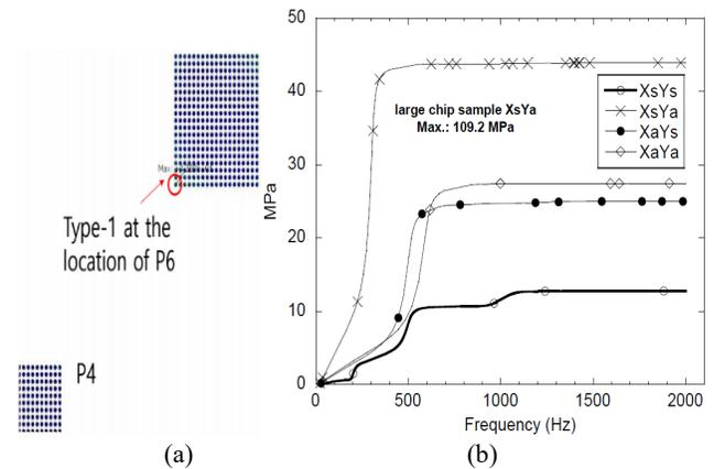
Figure 7. (a) Maximum solder stress location at Xs-Ya of the modified sample using 1/4 model. (b) The stress developments by changing the boundary conditions.
