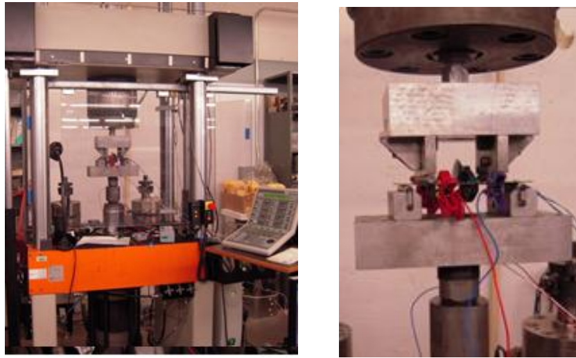
Figure 2. Four-point bend setup
