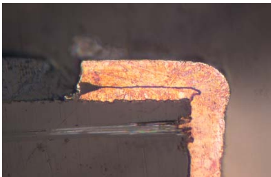
Figure 1: 200X notching after Ag Plate
