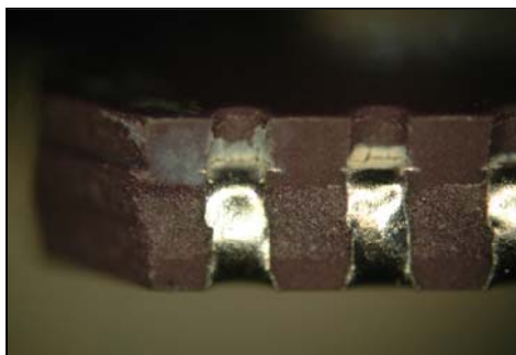
Figure 2. White residue in LCC castellations.
