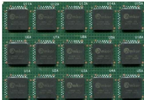
**Figure 5. Reliability test board**
