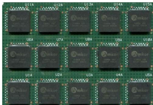
**Figure 5. Reliability test board**
