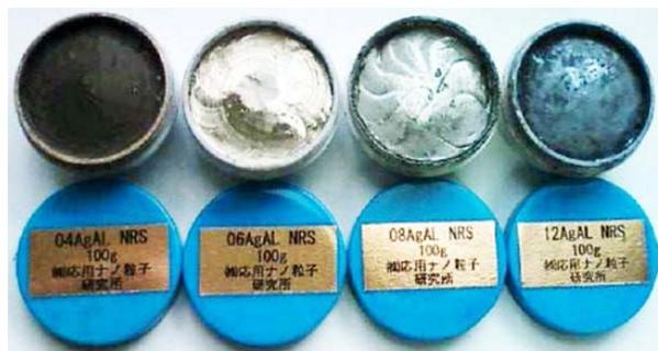
**Figure 20.** Examples of pastes based on alcoxide-stabilized nano-silver.
