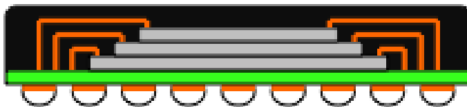
Figure 1. Progressively tiered die-stack and wire-bond package assembly.
