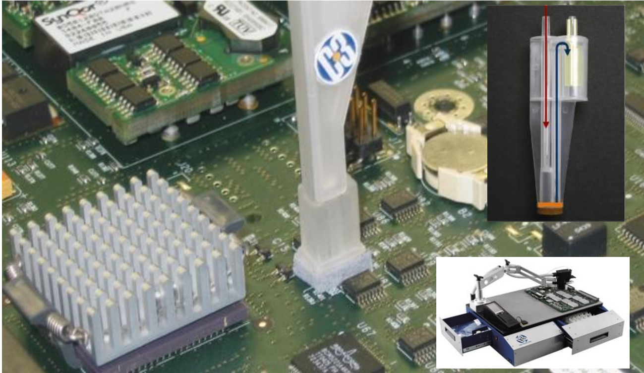
Figure 11 –Cleanliness test system
