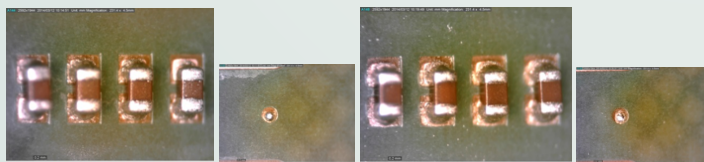
Figure 15. 0201 components and 6mil dot, water soluble Indium6.4 Type 6: ramp to peak left, soak right.
