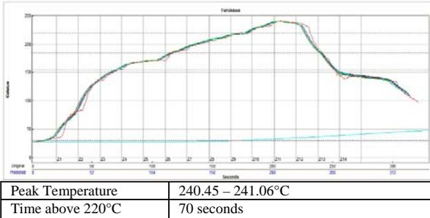
Figure 7: Reflow profile of SAC solder paste samples
