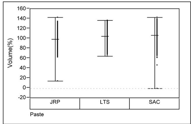
**Figure 3:** Post solder print volume distribution by paste
