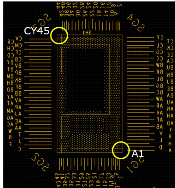
Figure 9: Top views of the package Land Pattern on the Mechanical Shock test Board with the monitored package corners shown by yellow circles.
