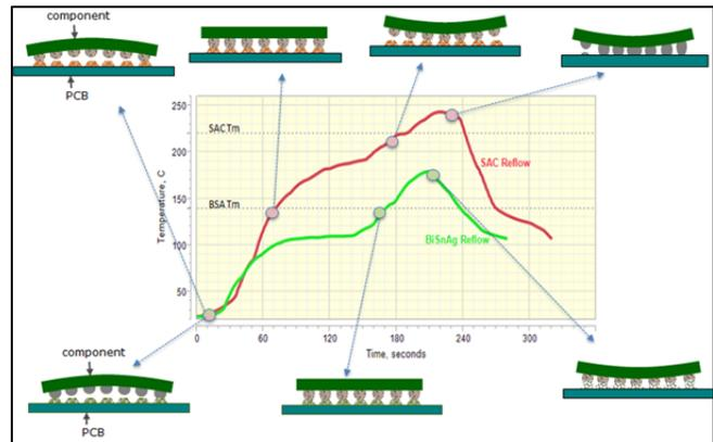
**Figure 1:** Comparison of typical warpage shapes of FCBGA packages during the reflow solder process for SAC and BiSnAg solder paste soldering Time-Temperature profiles
