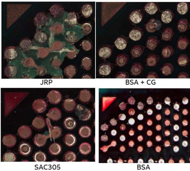
**Figure 13:** Dye and Pull Post Shock Failure analysis of JRP, BSA, BSA + CG and SAC305
