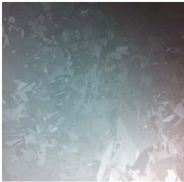
Figure 4. Polycrystalline Silicon Panel at 200 \mu\text{m} Thickness and 156mm x 156mm Panel Size
