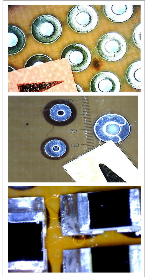
Fig. 13. Contamination embedded in base laminate on external layers bridging the insulation between pads, at outgoing inspection and after assembly.
