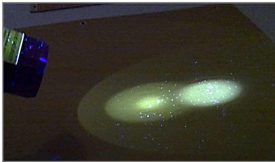
Fig. 12. Inspection of a sealed bag of polyimide prepreg showing UV fluorescence of particulate contamination.
