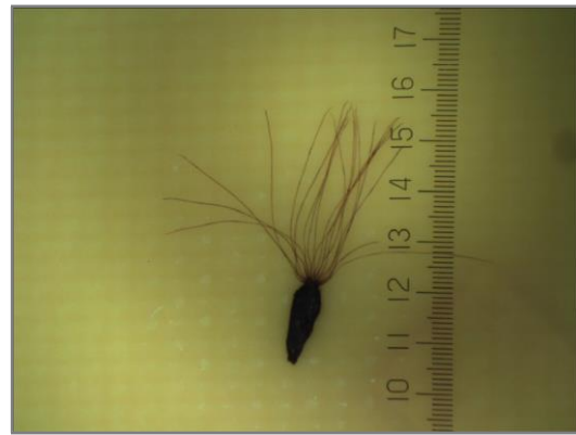
Fig. 8. Top view of a laminate after etching of copper cladding, showing a plant seed embedded in the dielectric material, probably carried into the clean room on clothes of personnel. The scale is in mm.
