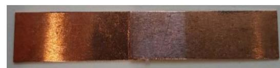
**Figure 2.** a) Schematic diagram of sample prepared for the tensile shear test, b) bonded copper foils sample
