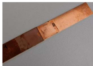
**Figure 12.** Fracture of the joints with spherical powder on the copper foil
