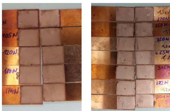
**Figure 11.** Fracture of the joints with a) spherical powder b) copper flake 1 and c) copper flake 2 on the copper foil
