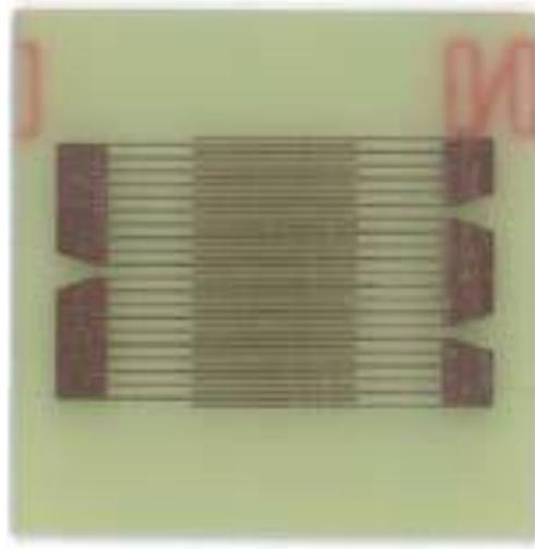
Figure 6: JIS SIR Test Board with 0.318mm line width and spacing
