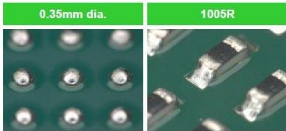
**Figure 18: Crack-free Paste A wetting/reflow test data for 0.35mm diameter board pads and soldered 1005R soldered chip components.**
