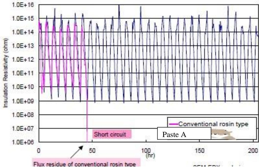
**Figure 10: Crack-free reflowed Paste A versus conventional reflowed Paste B during Dew Test method (A) testing**
