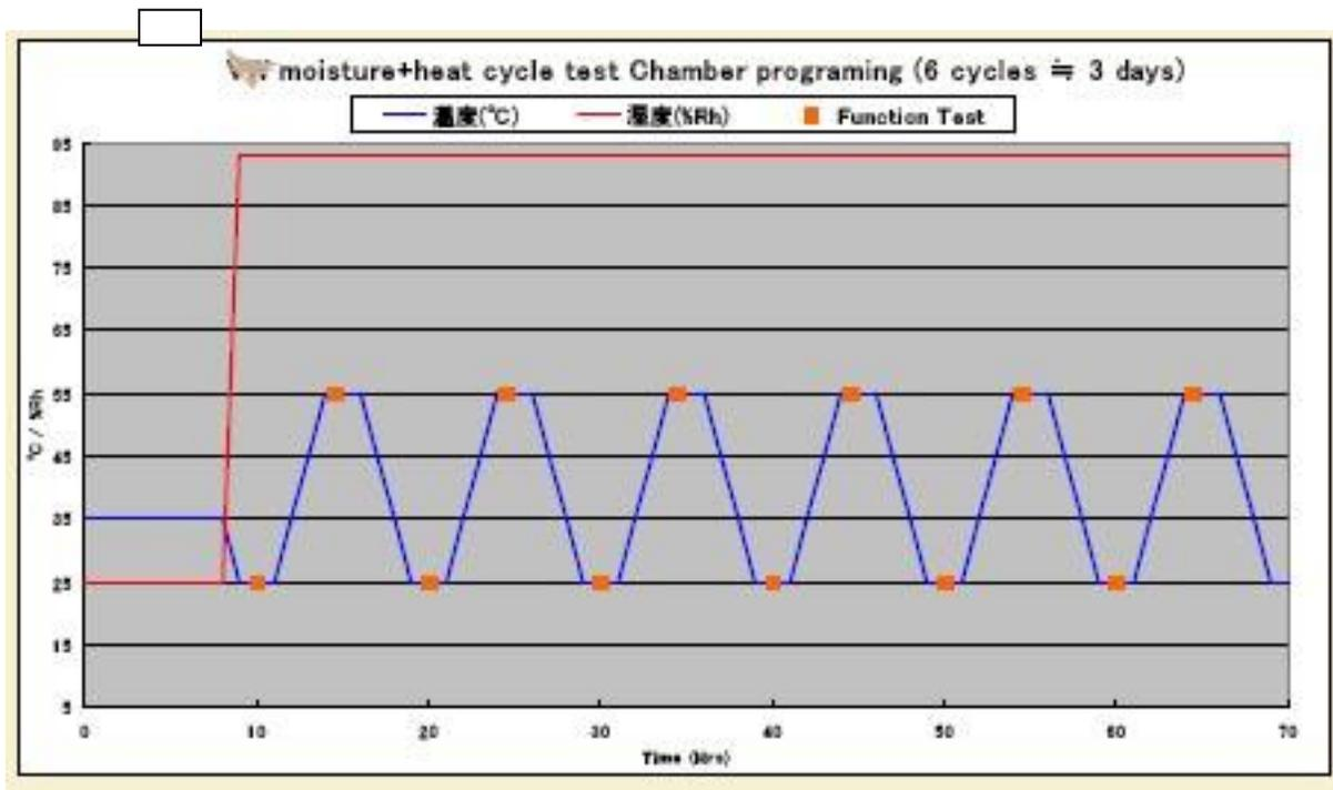
Figure 5: Dew Test Method (B) Temperature and Humidity Profile.
