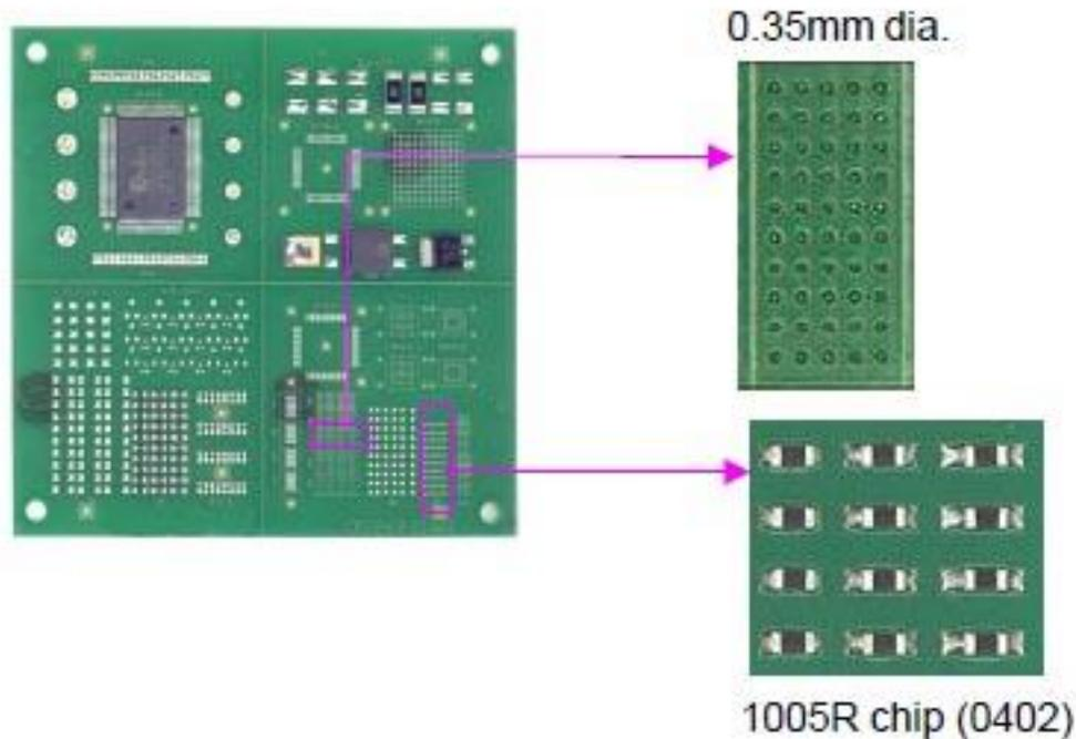
**Figure 7: Company Test Board for Wetting/Reflow Testing**
