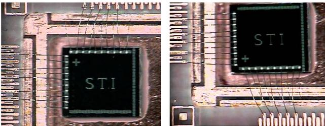
**Figure 2.** High-resolution images of daisy-chain die imbedded in the central cavity: upper left die (left) and lower left die (right).
