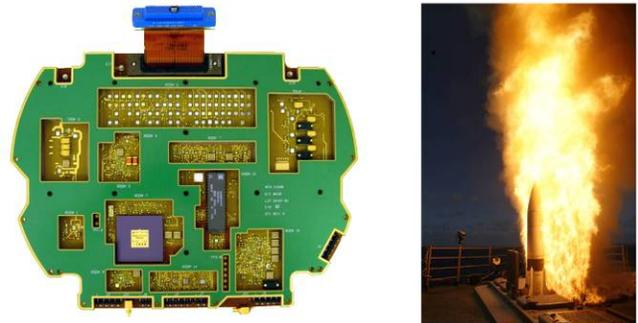
**Figure 4.** Mixed-signal prototype to demonstrate IC/DT® packaging technology’s capabilities (left) and successful test flight of prototype on SM-2 missile (right).
