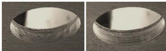
**Figure 3. Flexible PI PTH. Electroless copper (left) and electroless copper with stress reducing additives (right)**
