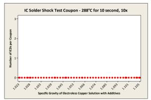
Figure 5. 10x Solder Shock test from a bath specific gravity of 1.02 – 1.10.
