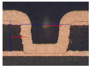
Figure 9. Cross section of an IST coupon MV after 1000 cycles.
