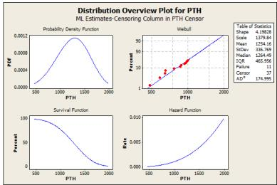
Figure 7. Distribution overview plot of all IST coupons based on cycles to failure. The data was right censored at 1000 cycles.
