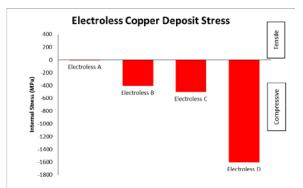
Figure 4. Electroless copper deposit stresses measured by spiral contractometer. Additives in the electroless copper solution have a significant influence on the resulting deposit stress.
