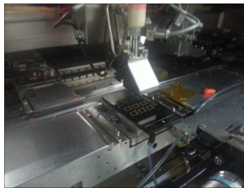
Figure 6: Flip chip bonding process.
