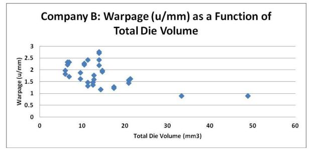
Figure 10 Company B: Component Warpage as a Function of Total Die Volume
