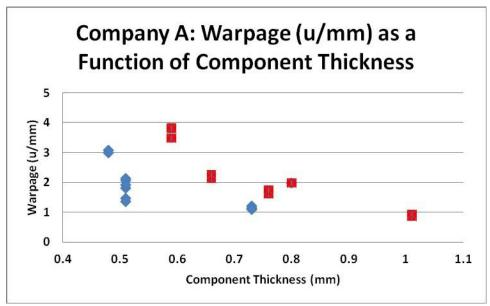
Figure 8 Company A: Warpage as a Function of Component Thickness, Highlighting Data Points of Components with Thicker Substrates
