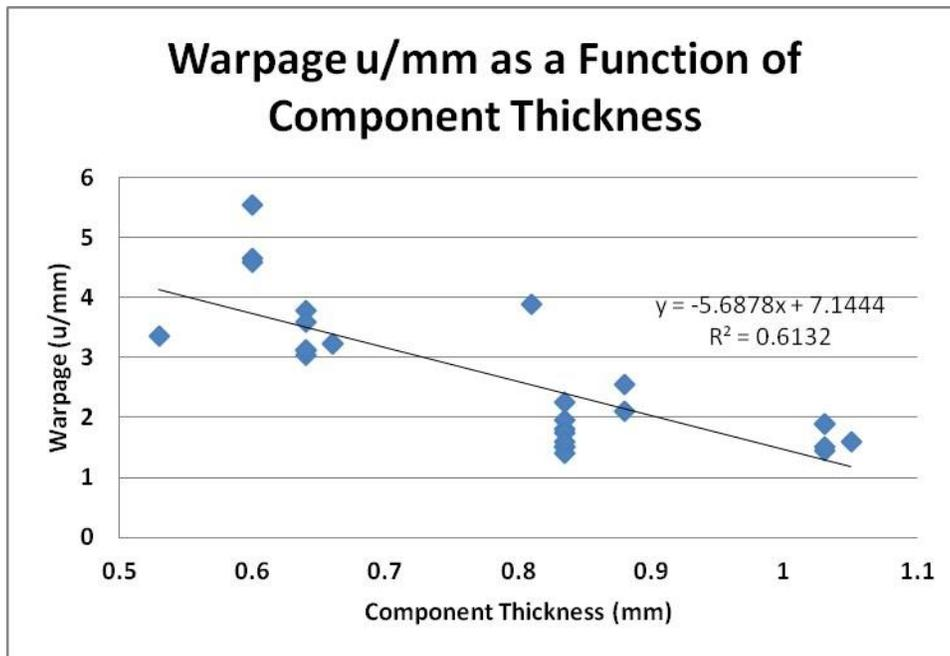
**Figure 4.** Warpage of Digital Components only as a Function of Component Thickness
