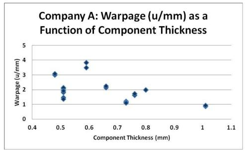
Figure 7 Company A: Warpage as a Function of Component Thickness
