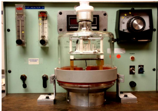
Figure 3 – A Glass Jar Soldering Unit Retrofitted with EA
