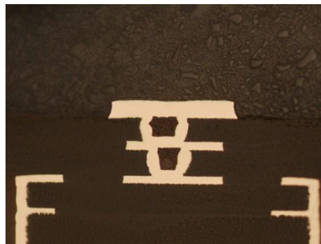
Figure 3 - Plugged and capped microvia 2]
