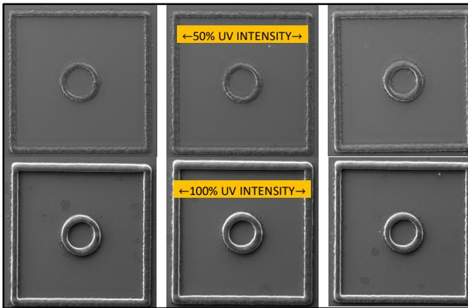
**Figure 36:** Effect of UV Intensity on the Via for ILD Ink-C
