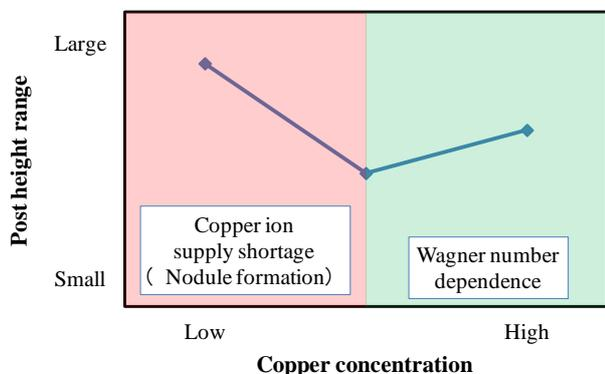
**Figure 10.** Influence of copper concentration on in-plane post height range
