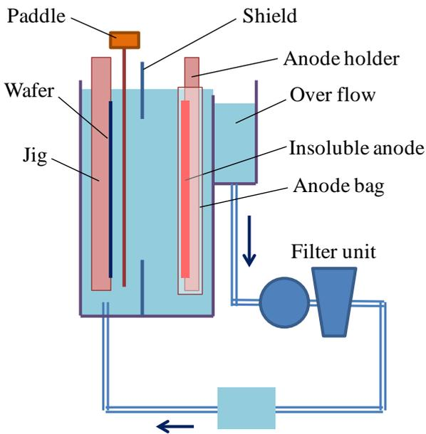
**Figure 2.** Paddle agitation plating equipment**Table 2.** Test conditions of post plating
