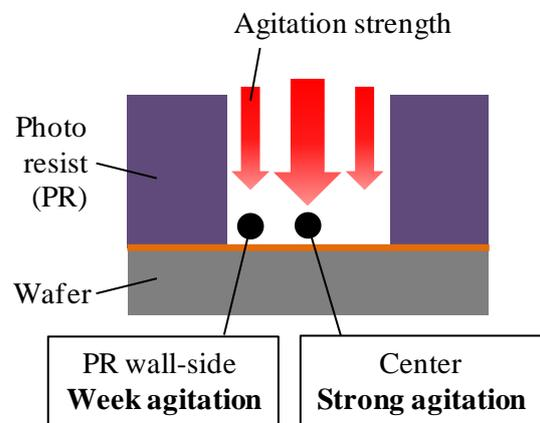
**Figure 3.** Agitation strength inside the PR opening
