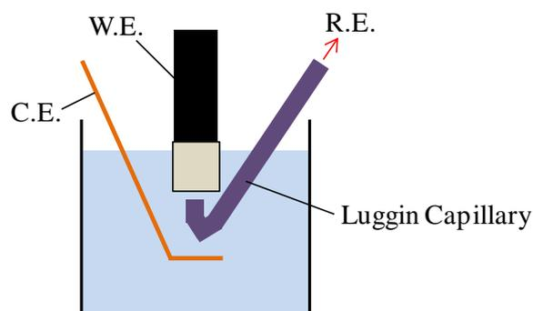
Figure 1. Three electrode system
