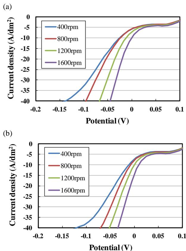
**Figure 5.** Influence of brightener concentration on polarization curve (a) Low brightener concentration, (b) High brightener concentration (Legend is rotation speed of disk electrode.)
