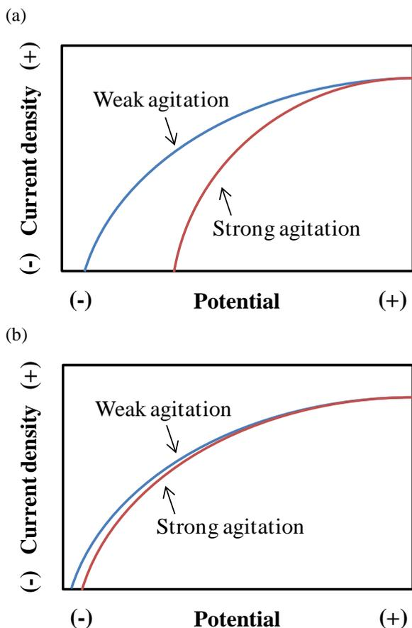
**Figure 4.** Relationship between polarization curve and post top shape (a) Convex shape, (b) Flat shape
