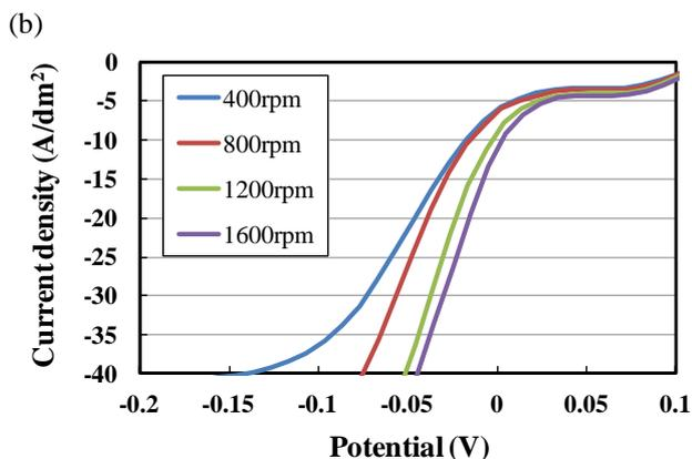
**Figure 6.** Influence of carrier concentration on polarization curve (a) Low carrier concentration, (b) High carrier concentration (Legend is rotation speed of disk electrode.)
