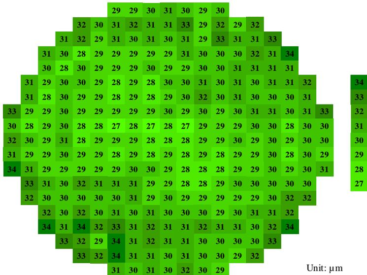
**Figure 11.** Post height distribution on 300 mm whole wafer (a) Average of post height (Each value was the average value within one chip), (b) Variation of post height (Each value was the difference between the maximum value and the minimum value within one chip)
