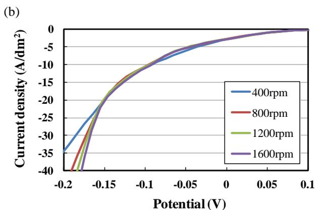
**Figure 7.** Influence of leveler concentration on polarization curve (a) Without leveler, (b) With leveler (Legend is rotation speed of disk electrode.)
