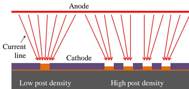
**Figure 9.** Influence of post density on current line distribution
