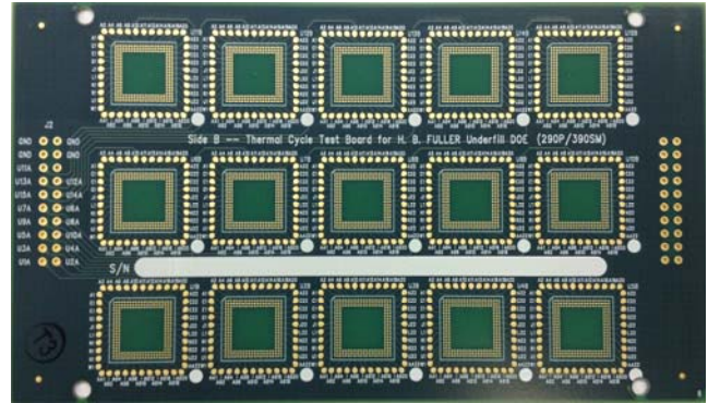
Figure 3: Test vehicle for reworkable underfill evaluation
