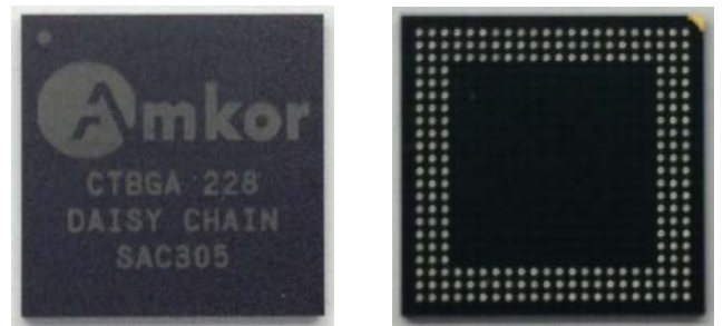
Figure 4: Device used in the reworkable underfill evaluation
