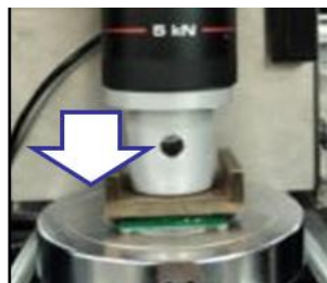
Figure 9 – Photo of the compression test setup
