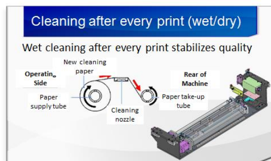
Figure 18 – Examples of Recommended Mask Cleaning Features
