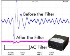
Figure 9. Reduction of noise on AC power line using stand-alone AC Filter
