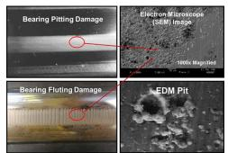
Figure 8. Damage to bearings due to high-frequency currents<sup>6</sup>
