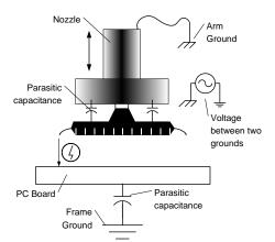
Figure 6. High-frequency current path through the device in pick-and-place
