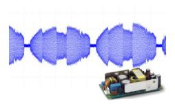
Figure 3. Noise on AC mains generated by several switched mode power supplies
