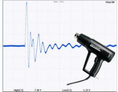
Figure 1. Power line transient from turning on heat gun.
