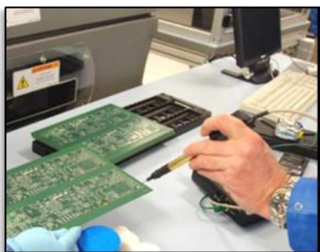
Figure 4. Measuring PC conductor with a high impedance contact volt meter
