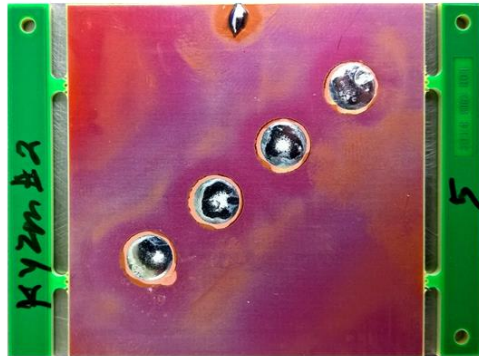
Figure 16: Image of Test Sample(s) measured with a Flat Cell
