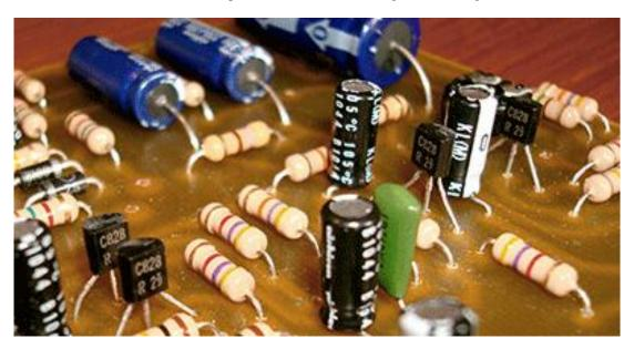
Figure 1: Carbon Resistors (as noted by their color rings)
