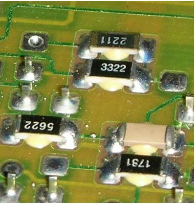
Figure 2: Surface Mount Resistors
