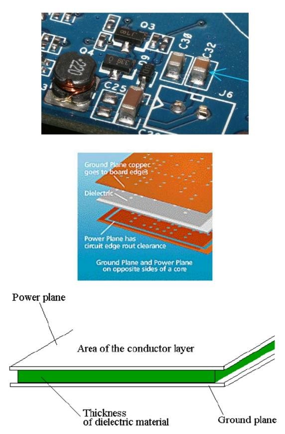
Figure 6: Various Capacitor evolution, ceramic paper, SMT and buried capacitive cores
