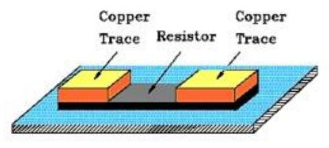
Figure 3: Thin Film Embedded Resistor
