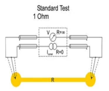
Figure 5: Resistor Measurement with Current Limiting
