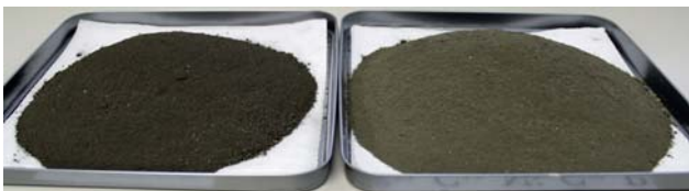
Figure 17. Oxide powder left after sweating out unoxidized solder from dross collected from SnCuNiGe (left) and SnCuNiGe+P (right).
