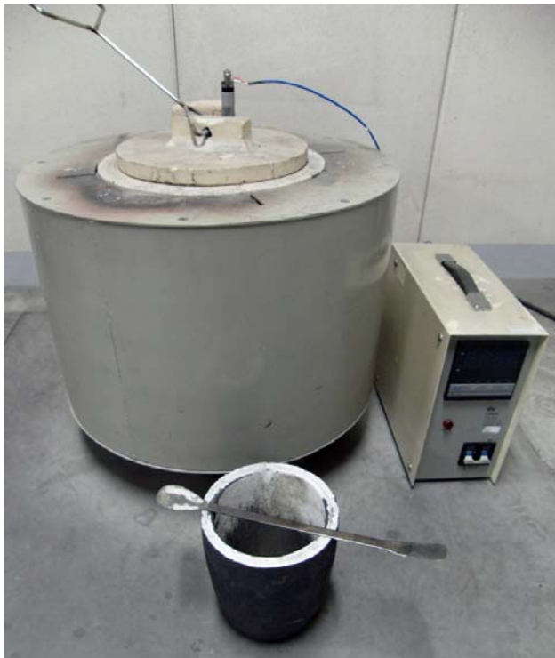
Figure 16. Crucible and furnace for sweating of dross to separate powder oxides from unoxidized solder.
