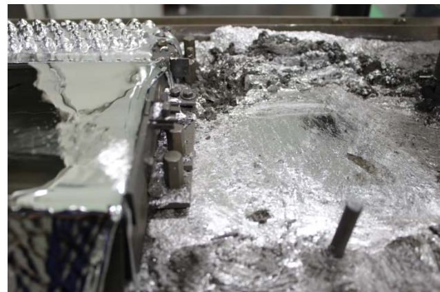
Figure 14. Dross accumulated on SnCuNiGe alloy after 8 hours operation at 255°C.
