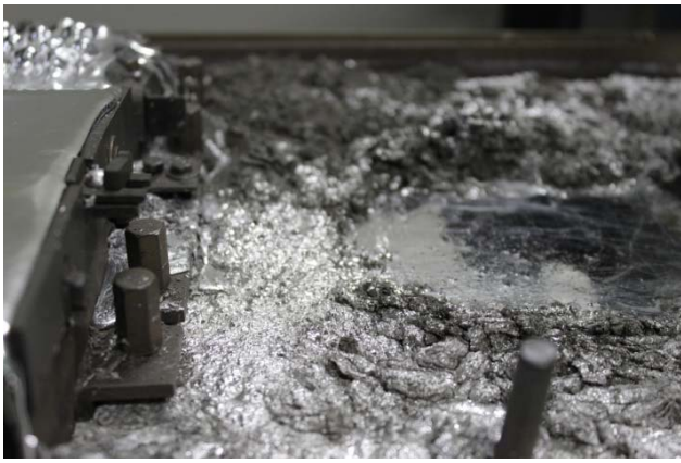
Figure 15. Dross accumulated on SnCuNiGe+P alloy after 8 hours operation at 255°C.
