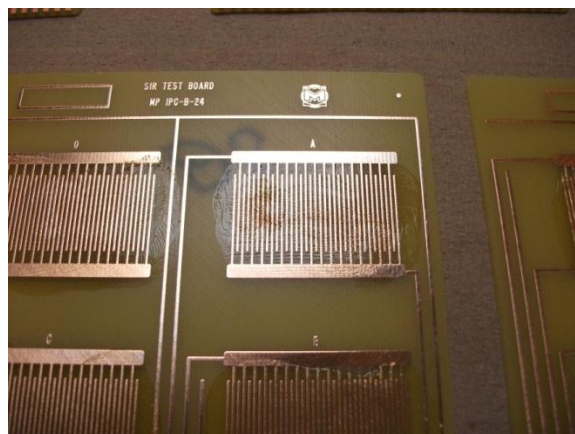
Figure 8 – Pizza Grease on SIR comb pattern as it appeared before or without a reflow cycle
