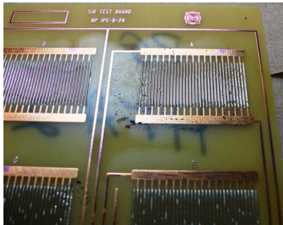
Figure 18 – Pizza Grease with Reflowed Solder Paste
