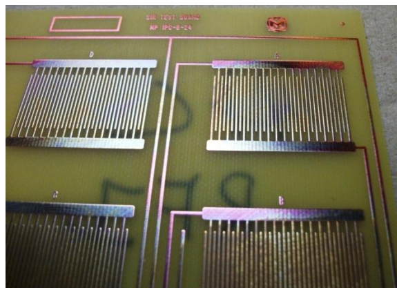
Figure 14 – Hand Cream on SIR comb pattern as it appeared after exposure to one reflow cycle (visible discoloration)
