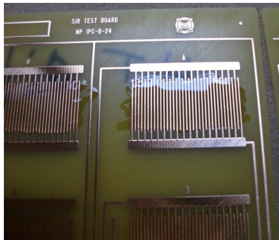
Figure 7 – High Temperature Reflow Chain Oil on SIR comb pattern as it appeared before or without a reflow cycle
