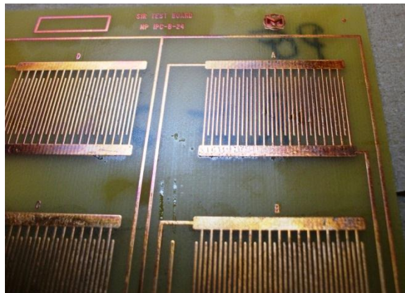
Figure 13 – Pizza Grease on SIR comb pattern as it appeared after exposure to one reflow cycle
