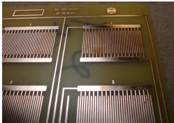
Figure 10 – Dried Tap Water on SIR comb pattern as it appeared before or without a reflow cycle (visible light staining)
