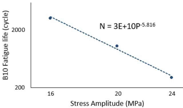
**Figure 11:** B10 versus stress Amplitude for SAC 305 solder joints without aging
