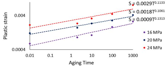
**Figure 18:** Plastic versus aging time for SAC 305 solder joints at different stress amplitudes
