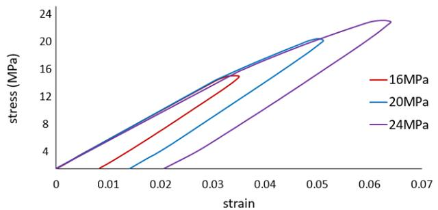
**Figure 15:** The hysteresis loops for SAC305 solder joints without aging in the steady state region for different stress amplitudes.
