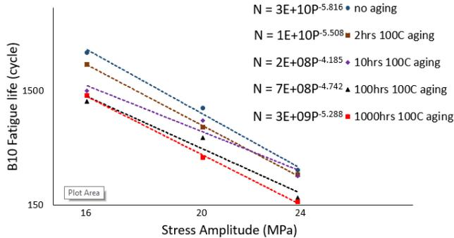
**Figure 12:** B10 versus stress Amplitude for SAC 305 solder joints under different aging times
