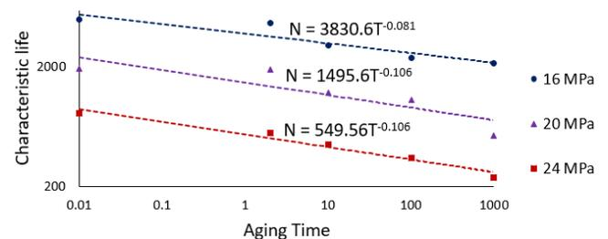
**Figure 10:** Characteristic life versus aging time for SAC305 solder joints under different stress Amplitudes
