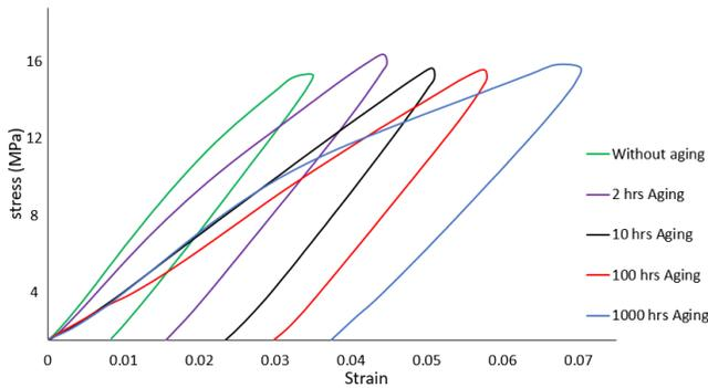
**Figure 16:** The hysteresis loops for SAC305 solder joints in the steady-state region for different aging times at 16 MPa stress amplitude.
