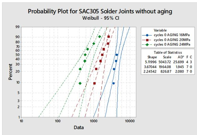
**Figure 5:** Two-parameter Weibull distributions for SAC305 without aging for different stress amplitudes
