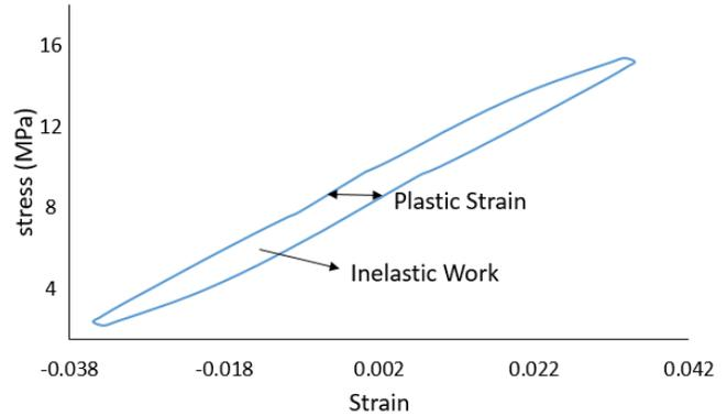
**Figure 13:** The full hysteresis loop for SAC305 solder joints without aging at 16 MPa stress amplitude.
