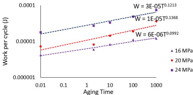
**Figure 17:** Inelastic work per cycle versus aging time for SAC305 solder joints at different stress amplitudes
