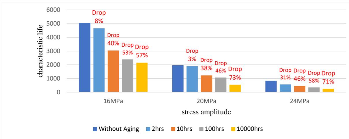
**Figure 7:** The characteristic life and the percentages of reduction in the characteristic life for lead-free SAC305 solder joints under different aging times
