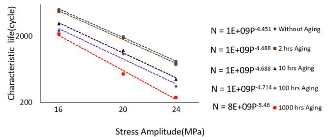
**Figure 9:** Characteristic life versus stress Amplitude for SAC 305 solder joints under different aging times
