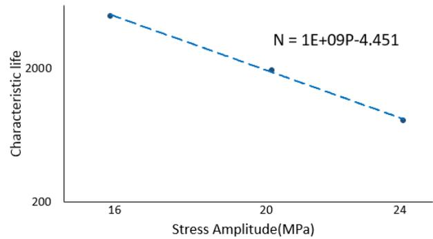
**Figure 8:** Characteristic life versus stress Amplitude for SAC305 solder joints without aging
