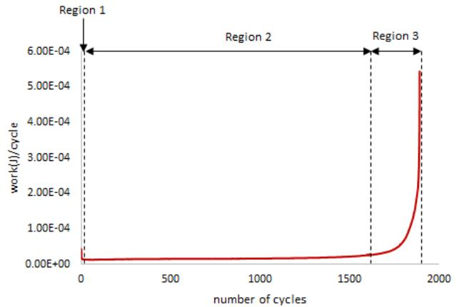
**Figure 14:** Inelastic work versus the number of cycle for SAC305 solder joints without aging cycled at 20 MPa stress amplitude.
