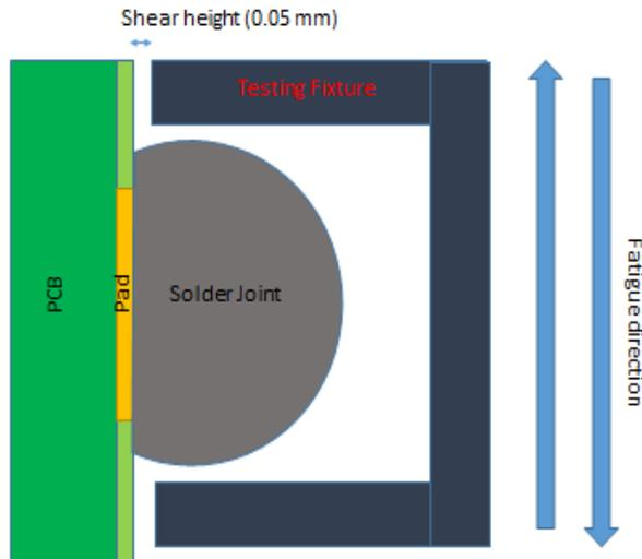
**Figure 4:** Schematic of the cylindrical testing fixture for individual solder joint
