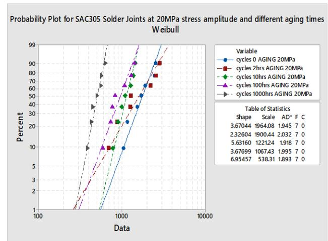
(b) Two-parameter Weibull distributions under 20 MPa stress amplitude and different aging times
