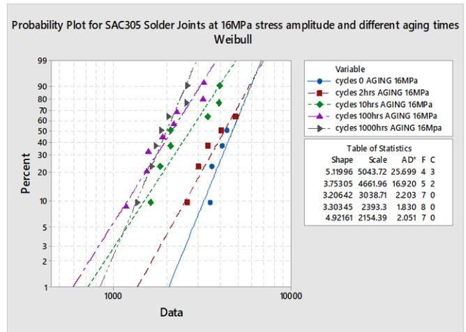
(a) Two-parameter Weibull distributions under 16 MPa stress amplitude and different aging times
