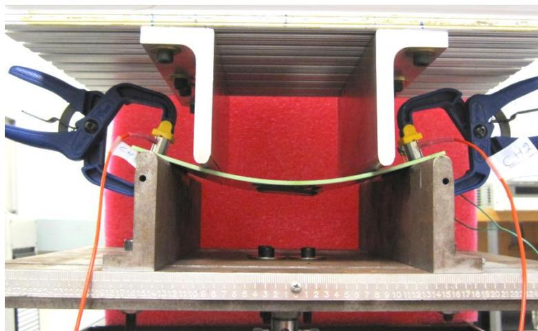
**Figure 4 - Four Point Bend Testing of HSBGA board**
