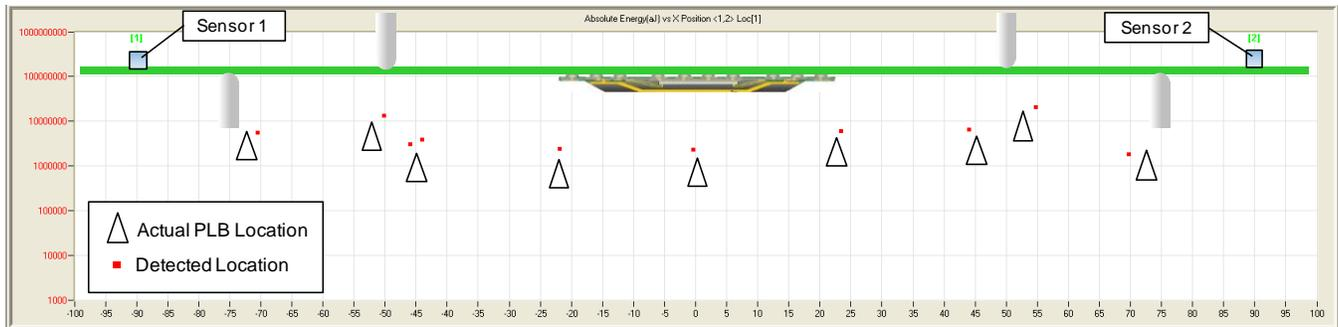
**Figure 5 - Linear Source Location Using PLB Test for HSBGA Boards**
