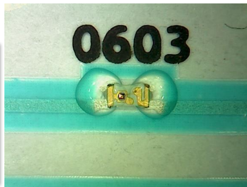
Figure 10. Robust SMT Joint Design
