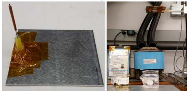
**Figure 6:** Wire Test Fixture (left), Fixture Installed on Test Dipping Apparatus (right)
