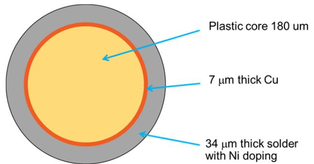
**Figure 2.** Construction of 260 μm plastic core ball.
