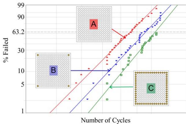
**Figure 12.** TC Weibull Plots For Three Plastic Core Ball Placement Options.
