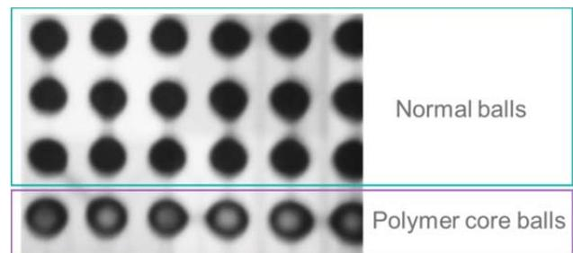
**Figure 9.** Appearance of plastic core ball joints in comparison with normal solder joints.
