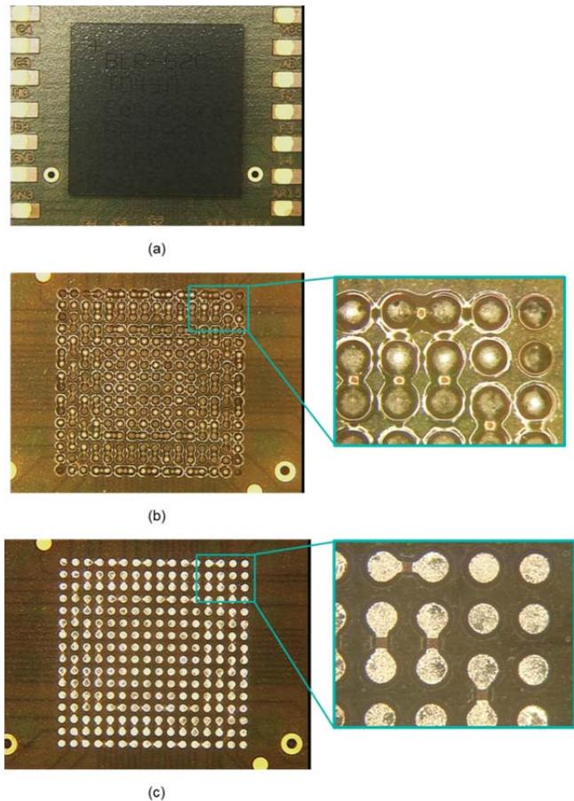
**Figure 11.** Pictures of the Test Boards during Board Rework of A WLP with Plastic Core Balls. (A) Before Rework, (B) After WLP Removal, And (C) After Site Dressing.
