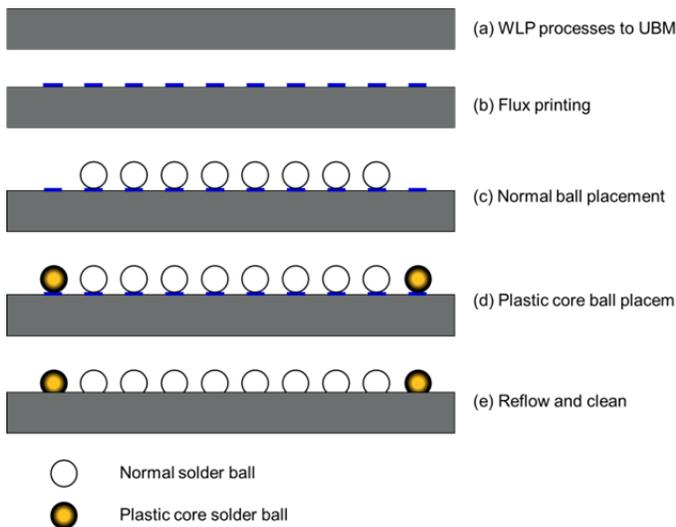
**Figure 5.** Manufacturing Process Steps of WLP with Plastic Core Balls.
