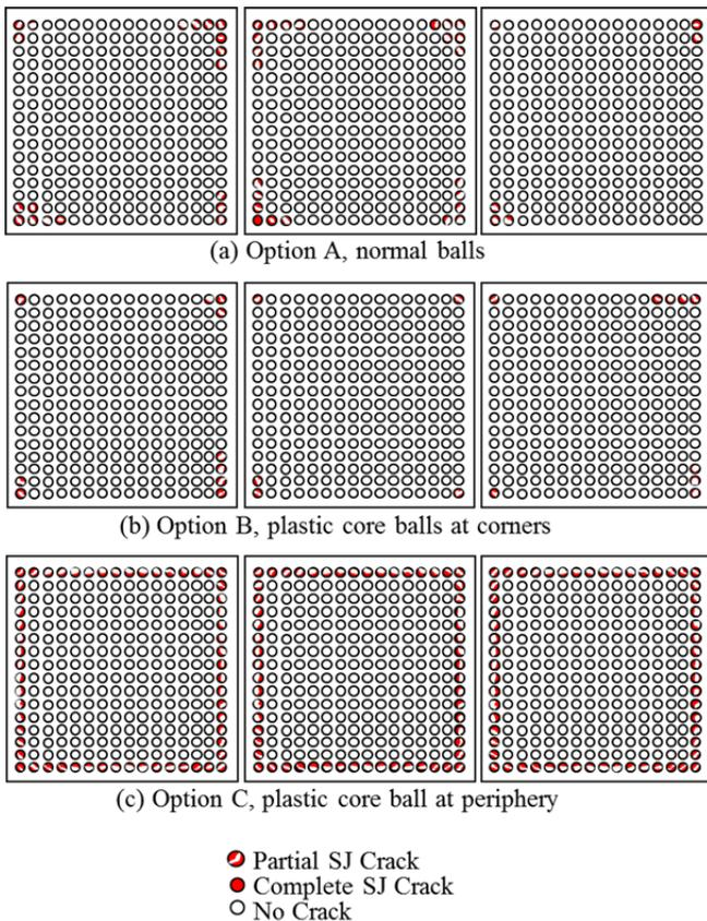
**Figure 15.** Solder Joint Crack Map Of Units Subjected To A Given TC Duration
