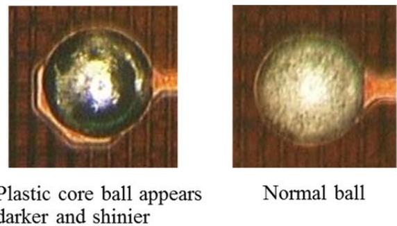
**Figure 8.** Plastic Core Ball Appearance In Comparison With Normal Balls.
