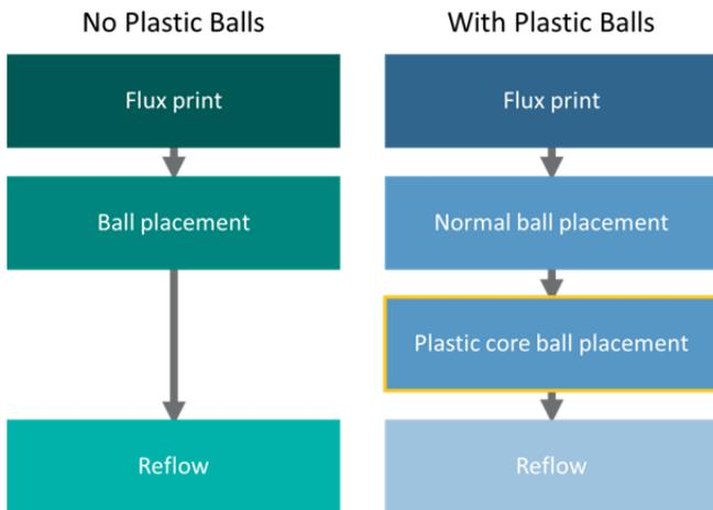
**Figure 6.** Ball placement process comparison between single and mixed ball types.
