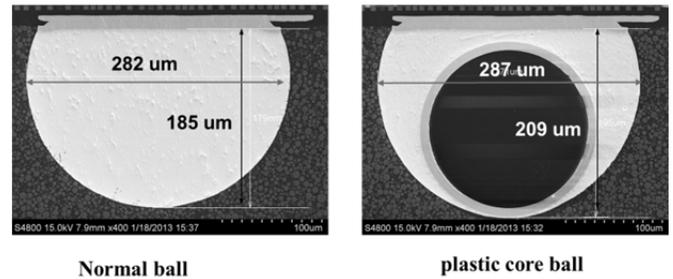
**Figure 7.** Comparison of Solder Height between a Normal Ball and a Plastic Core Ball.
