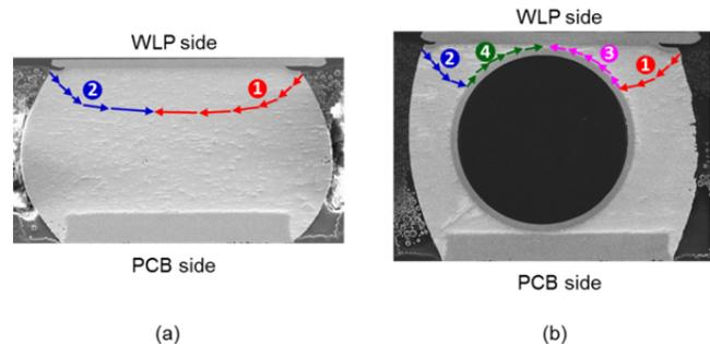
**Figure 14.** Illustration Of Solder Joint Crack Propagations. (a) Normal Solder Joint, And (b) Plastic Ball Solder Joint.
