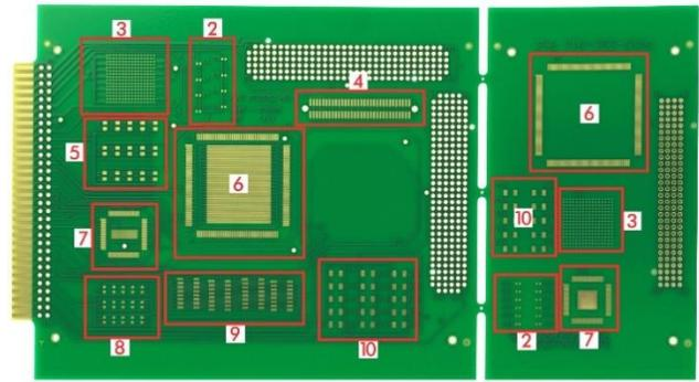
**Figure 17.** IPC-B-52 Test Coupon (SIR mini-coupons not used)
