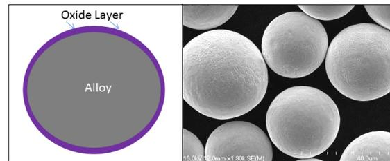
**Figure 3.** Solder Powder Oxide Layer
