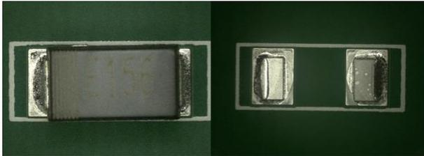
**Figure 15.** Type 4, Surface / Under-Component - 6032
