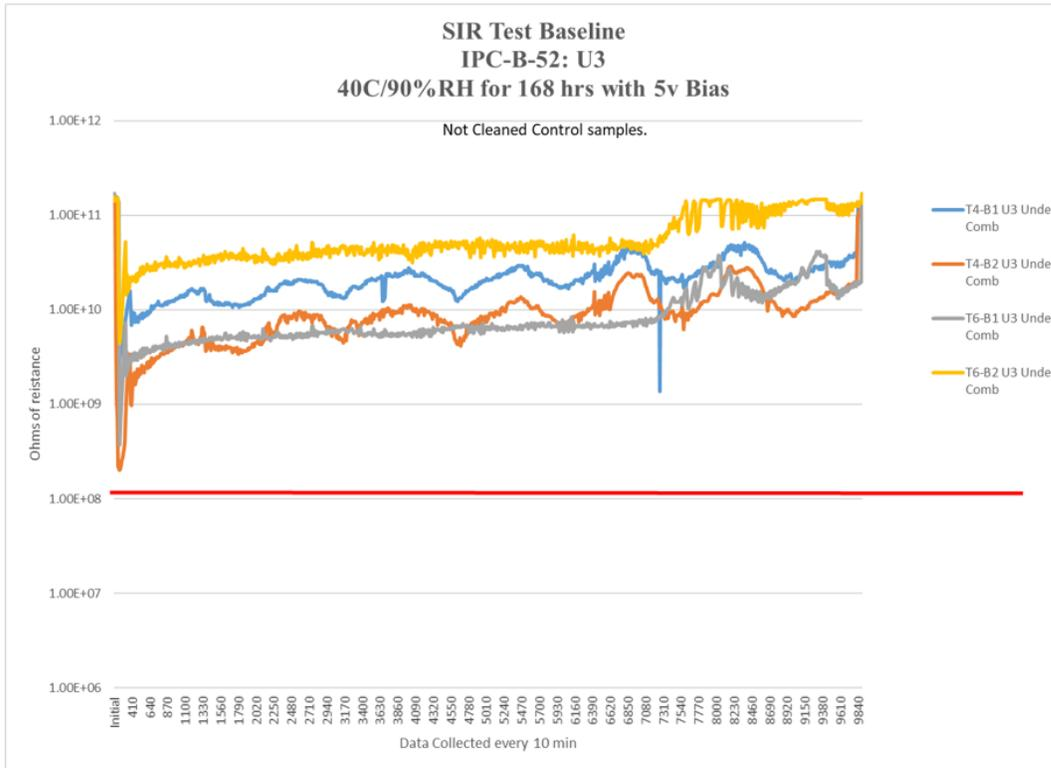
**Figure 28.** SIR Test Cleaning Trials 1-8 IPC-B-52: U3
