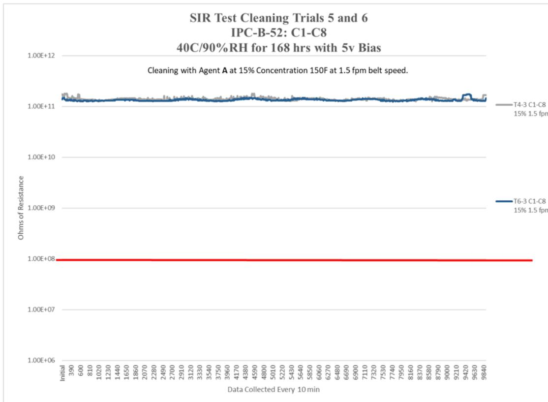
**Figure 30.** SIR Test Cleaning Trials 5 and 6: C1-C8
