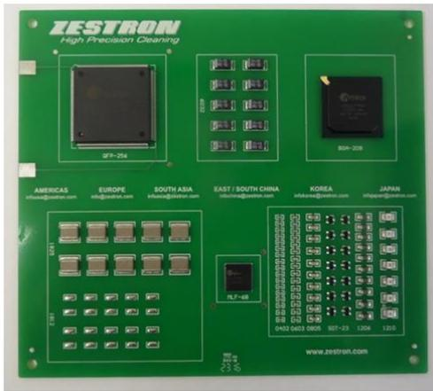
**Figure 4.** Fully Populated ZESTRON Test Vehicle
