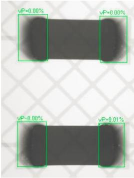
**Figure 20.** Solder Joint X-ray
