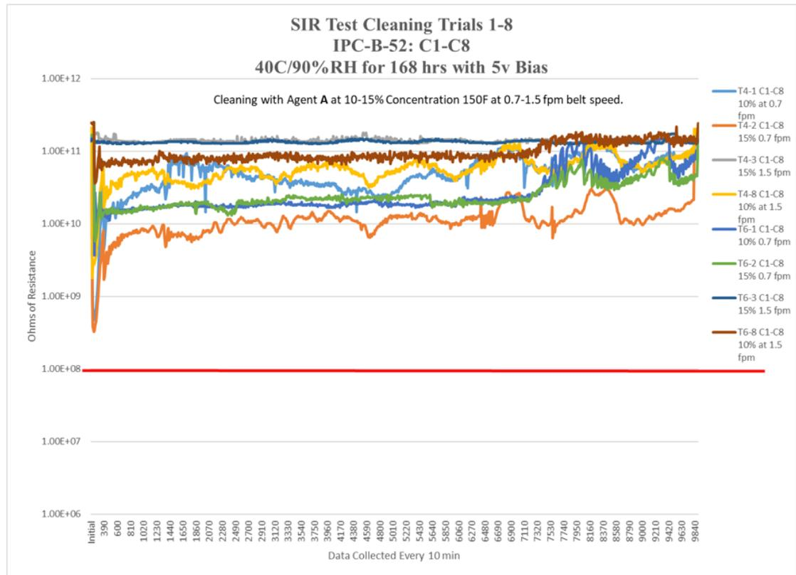
**Figure 25.** SIR Test Cleaning Trials 1-8: C1-C8
