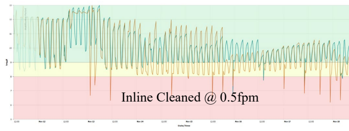
Figure 16: Channel C at 40°C / 90% RH / 5 V for 72-hours
