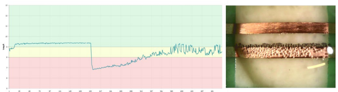
Figure 2: Leakage Currents resulting in No-Fault Failures
