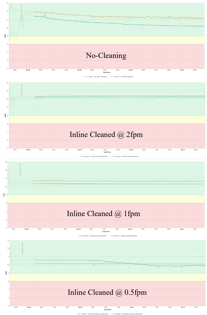
Figure 18: Channel D SIR @ 90% RH / 5V for 72-hours
