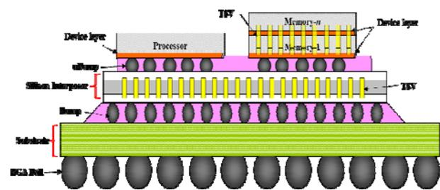
**Figure 1.** Schematic Drawing of 3D Stacking of the Silicon Interposer with TSV
