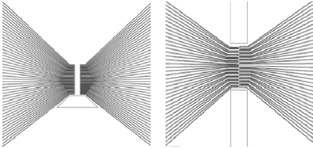
**Figure 3.** Illustrative Drawing of Two-layer Cu Interposer
