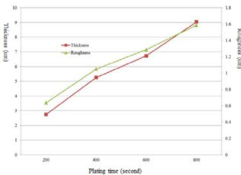
**Figure 8.** Variation of the Copper Thickness and Surface Roughness under 30mA of Plating Current
