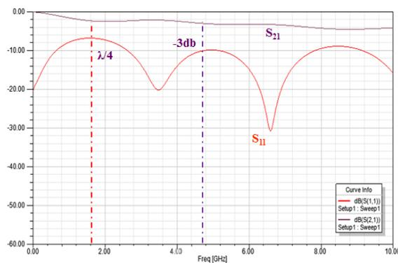
**Figure 4.** Simulation Results of the Frequency Dependent Scattering Parameters for the Structures depicted in Figure 3
