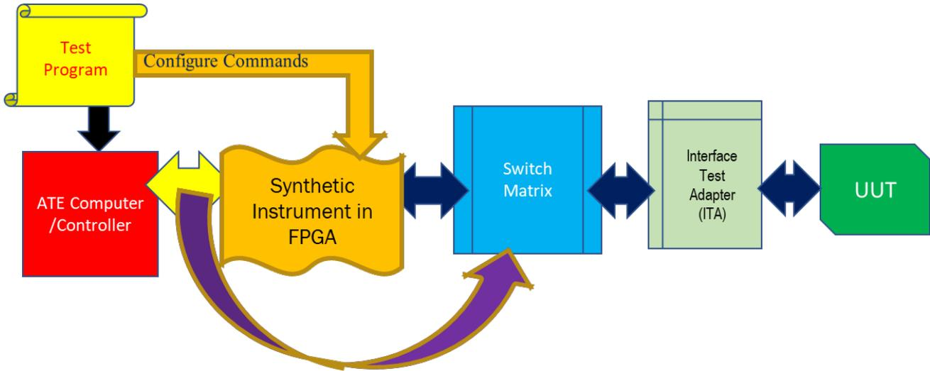
**Figure 2–A Synthetic ATE consisting of a Synthetic Measurement System and Synthetic Instruments**
