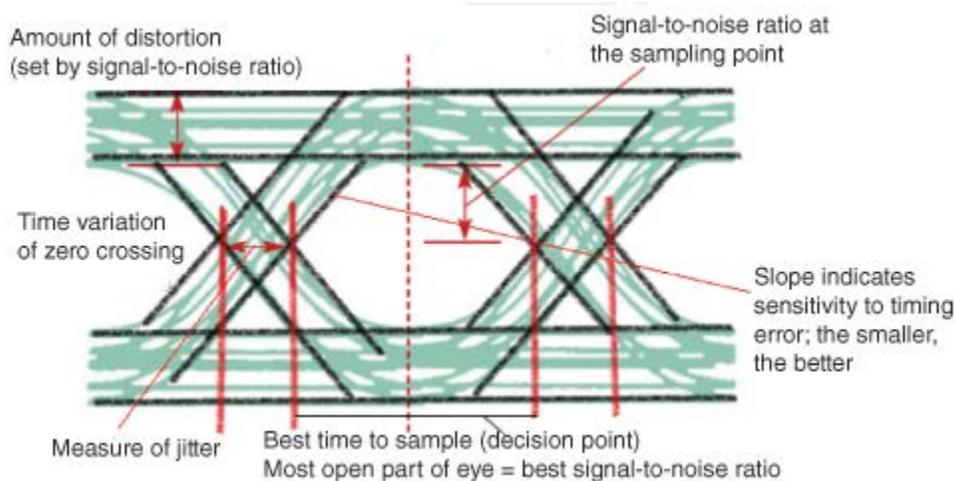
Figure 4 –An Eye Diagram and its Characteristics [10]
