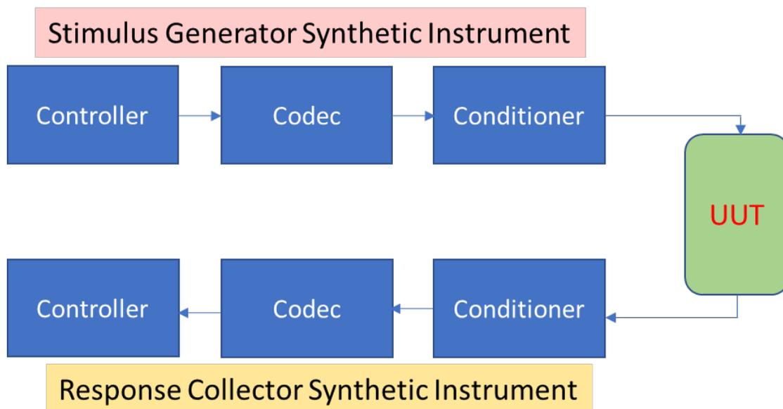
Figure 1 –Synthetic Instruments (SIs) in a Synthetic Measurement System (SMS) [9]
