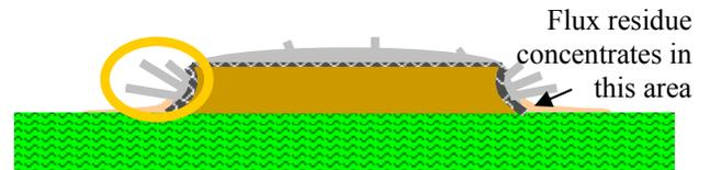
**Figure 5.** Schematic indication of pattern of whisker growth.
