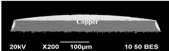
**Figure 2.** Cross-section of typical soldered trace
