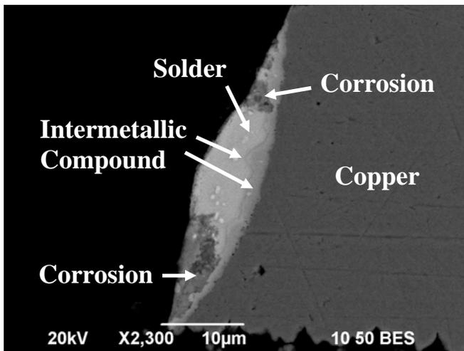
**Figure 3.** Cross-section of solder coating
