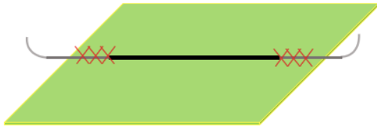
Figure 1. A schematic of a piece of fabric with MWCNT track and connection cables properly sewed to provide continuous connection between the fabric and the instrument.
