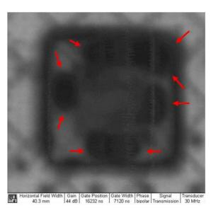
**Figure 7** - Through-scan mode of an underfilled QFN assembly. Large voids in the underfill (red arrows).
