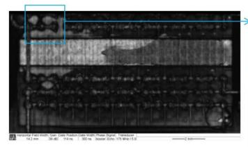
**Figure 12** - C-scan mode of an underfilled BGA assembly after micro-mechanical polishing. Evidence of a delaminated area
