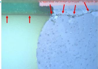
**Figure 13** - Optical view in cross-section of the underfill between solder joints: delamination at underfill/BGA interface generating cracks in the solder joints (red arrows)
