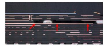
**Figure 4** - Through-scan mode of an underfilled board. Voids in the underfill under an LGA assembly (red arrows).
