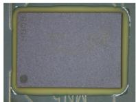
Figure 1 - Global view of an underfilled BGA
