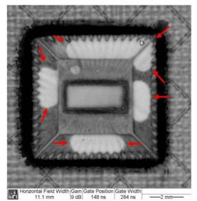
**Figure 6** - C-scan mode of an underfilled QFN assembly. Large voids in the underfill (red arrows).
