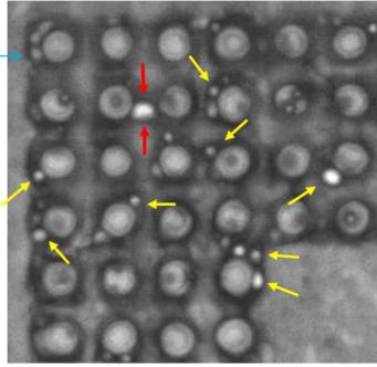
**Figure 10** - Detailed view of the underfill between solder joints: Voids in the underfill (yellow arrows) and void that encircles two solder joints (red arrows)
