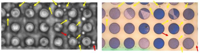
**Figures 11** - Same area of the underfilled BGA assembly after micro-mechanical polishing in C-scan mode (left) and in optical under polarized light after further planar polishing (right). Voids in the underfill correlated between C-scan and optical inspection (yellow arrows) and voids not detected optically in this planar axis (red arrows)
