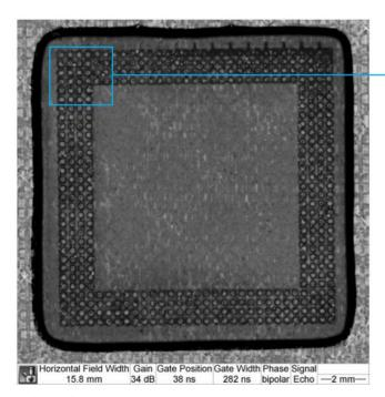
**Figure 9** - C-scan mode of an underfilled BGA assembly after micro-mechanical polishing.
