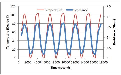
Figure 1. Resistance is a function of temperature.
