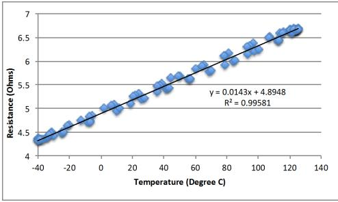
Figure 10. Resistance is a function of temperature
