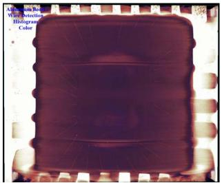
**Figure 7.** CT Image Showing Aluminum Bond Wires Inside a Package Utilizing a Color Scale Histogram
