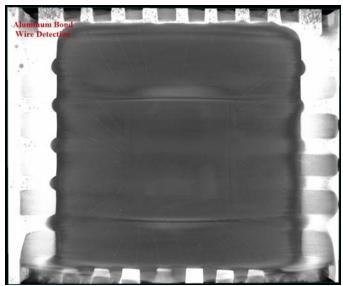
**Figure 6.** CT Image Showing Aluminum Bond Wires Inside a Package Utilizing the Black and White Histogram
