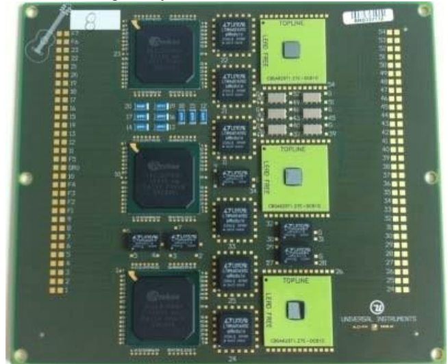
Figure 4: AREA test card used for HoP AXI inspection
