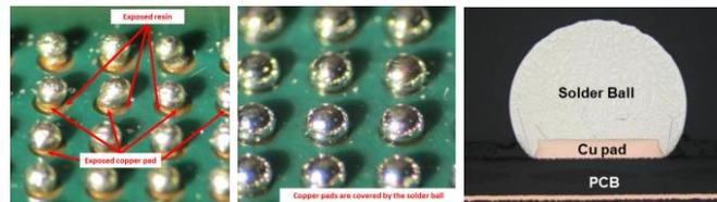
**(a) Reject (b) Accept (c) Cross-section joint**
