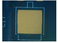
Figure 11: Wave Flux F (ActDry) Before Cleaning
