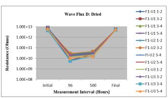
Figure 26: Wave Flux D – Dried Minimum Requirement: 1.57E+09 (Pass)
