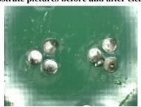
Figure 7: Wave Flux D (ActDry) Before Cleaning
