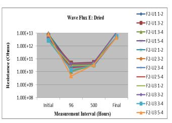
Figure 28: Wave Flux E – Dried Minimum Requirement: 2.24E+09 (Pass)
