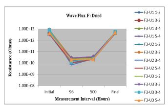
Figure 30: Wave Flux F - Dried Minimum Requirement: 1.68E +09 (Pass)
