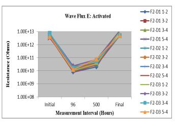
Figure 27: Wave Flux E – Activated Minimum Requirement: 1.32E+09 (Pass)
