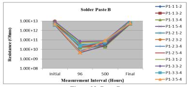
Figure 23: Paste B Minimum Requirement: 1.88E+09 (Pass)
