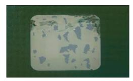
Figure 34: After Cleaning - Varnish removed after five passes through the inline cleaner
