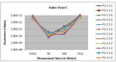
Figure 24: Paste C Minimum Requirement: 1.33E+09 (Pass)
