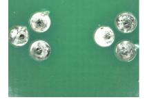
Figure 8: Wave Flux D After Cleaning
