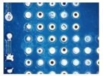
Figure 9: Wave Flux E (ActDry) Before Cleaning
