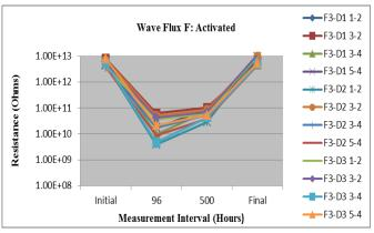
Figure 29: Wave Flux F - Activated Minimum Requirement: 1.86E+09 (Pass)
