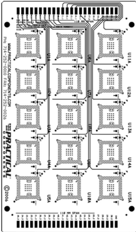
Figure 1. PoP 14mm test board
